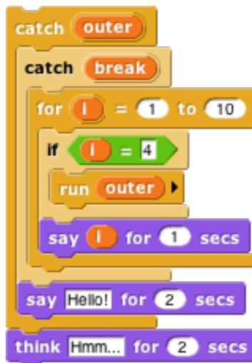
As shown, this will say 1, then 2, then 3, then exit both nested **catch**s and think “Hmm.” If in the **run** block the variable **break** is used instead of **outer**, then the script will say 1, 2, 3, and “Hello!” before thinking “Hmm.”
